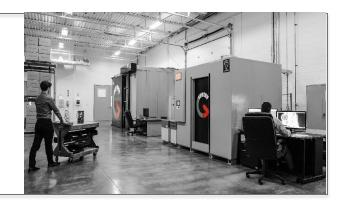
Advanced manufacturing at our facility relates to the **internal** inspection of parts and assemblies using computed tomography. This would be either for failure investigation, new product validation, and production inspection for high value – low volume parts.
