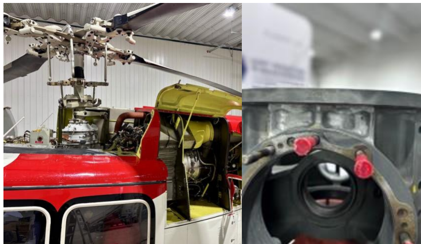
Figure 11 Polycontrols cold spray capability allowed a novel gearbox repair to be validated for a Canadian aerospace overhaul customer
