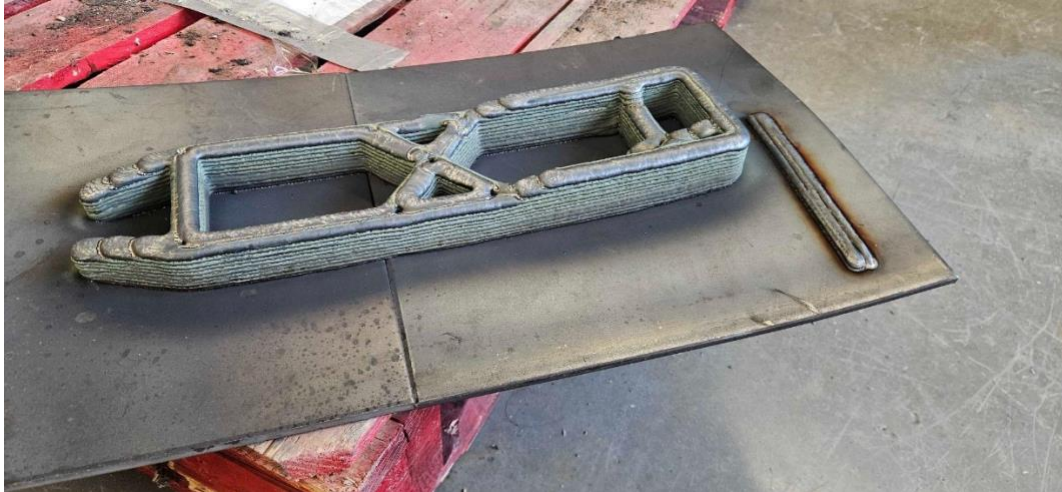
Figure 19 Elementiam WAAM printing of near-net-shape stock (Fronius MIG welder, Yaskawa collaborative robot, Element X software)
