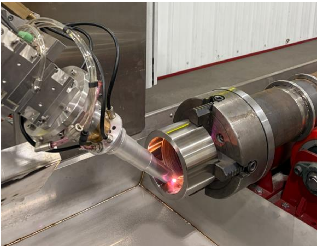
Figure 13 Apollo-Clad developed a novel process for maritime applications, using sacrificial tubes to add Nickel Aluminum Bronze and efficiently produce large shafts
